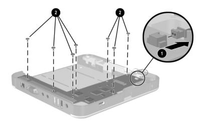
Removing the Board Assembly Screws
